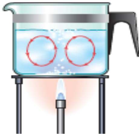
Figure 19 The flame heats water at the bottom of the pot. The warm water rises, then as it cools, it sinks back down.
